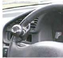
Steering Ball can provide postural options...suitable for fitting to steering wheels of tractors and other vehicles.
